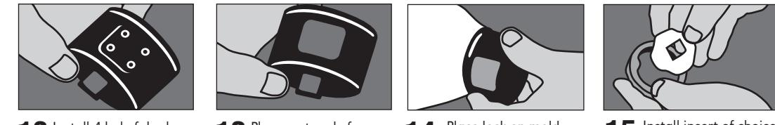
12 Install 4-hole fab plug. Snug tighten screws only DO NOT over-torque.
