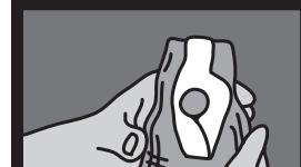
**44** Reinforce with carbon tape between posts. Avoid extra material around fabrication plug for easier removal.
