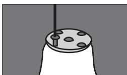
**45** Lubricate screws and install five hole plate. (See Caution #4)
