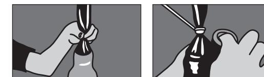
**47** Pull bag and laminate. Initially restrict flow to force lamination through center hole on plate to force out air pockets.
