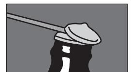
**50** Expose edge and remove excess lamination.
