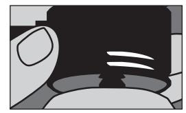
**1** Install pin on liner. Engage lock to check for play between lock and liner.
